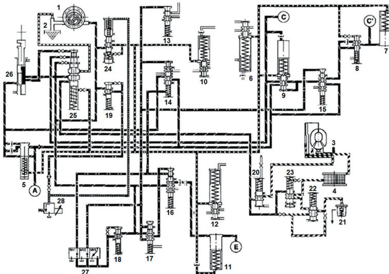
Fig. 3. Structural model of internal leakage in the electrohydraulic AT controller in the configuration of the 2<sup>nd</sup> gear (for the meaning of the reference numbers of individual components of the hydraulic control system see Fig. 1) [13]
