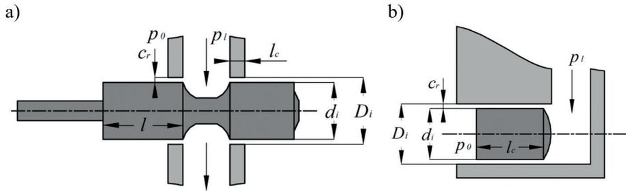
Fig. 4. Schematics of precision hydraulic pairs in an electrohydraulic controller: a) spool distribution valve; b) hydraulic damper;  $p_0$ ,  $p_i$  – pressures;  $l$  – length of the cylindrical part of the spool
