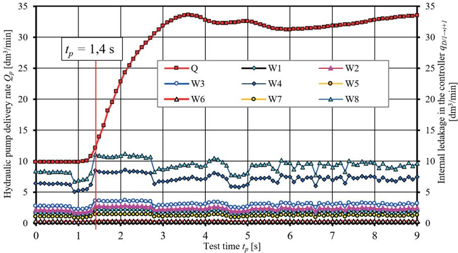
Fig. 8. Time history of the internal leakage rate  $q_{D/I \rightarrow I+1}$  in the electrohydraulic controller in the conditions of the minimum vehicle acceleration test in gears "1" and "2", for the calculation variants from W1 to W8
