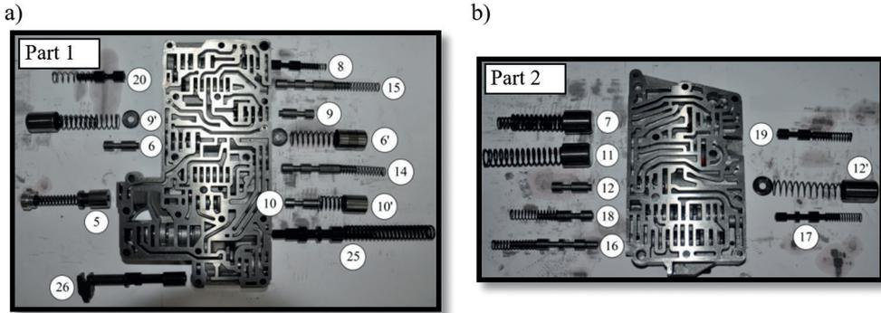
Fig. 6. Electrohydraulic controller blocks: a) Part 1; b) Part 2
