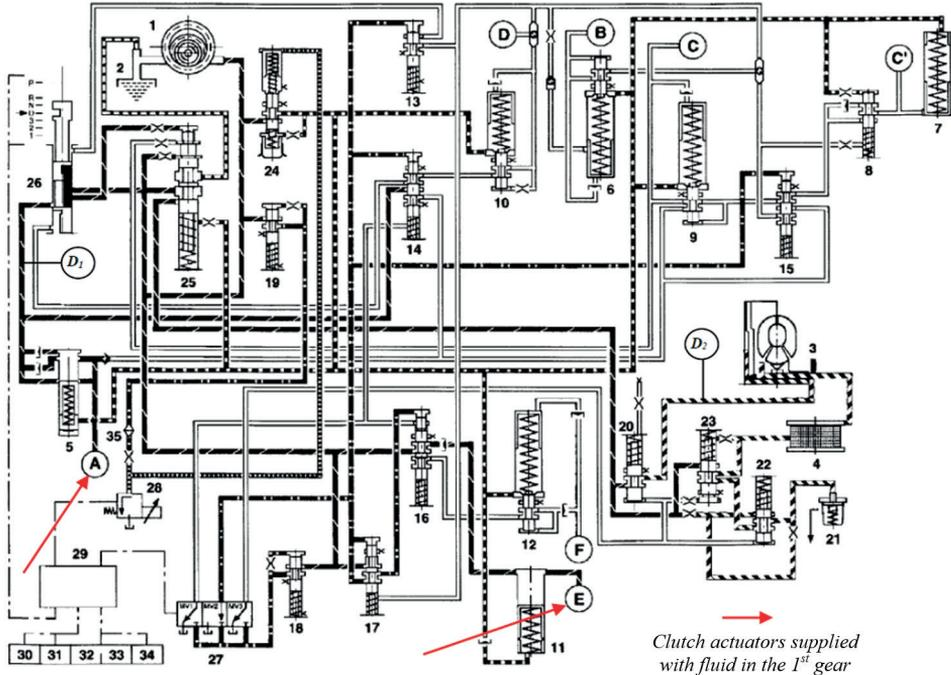
Fig. 1. Schematic diagram of the hydraulic control system of the ZF4HP-24 automatic transmission, with the ATF flow routes having been shown for the selector lever being set to "D" and for the 1st gear being implemented:
