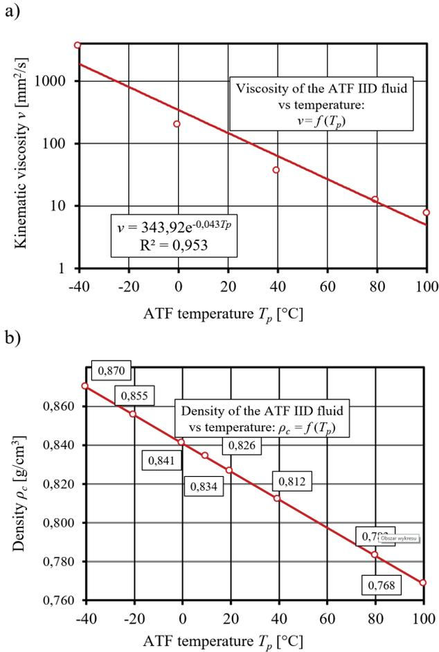
Fig. 7. Characteristics of the ATF IID fluid vs temperature:
