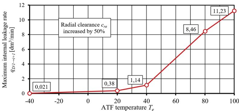
Fig. 9. Maximum values of the rate of internal leakage  $q_{D/I \rightarrow i+1}$  in the electrohydraulic controller vs ATF temperature  $T_e$  for the test conditions covering drive in gear "1", acceleration, "1→2" gearshift process, and drive in gear "2", with an assumption of significant wear of the interfacing surfaces of the precision hydraulic pair (i.e. with the radial clearance values  $c_{re}$  increased by 50 %)
