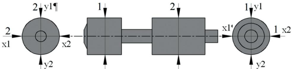
Fig. 5. Schematic presentation of the diameter measurement places for the spool of distribution valve 6 (reference number as shown in Figs 1 and 3)
